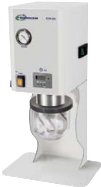
**ECM 300** - For plasters and investments. Possibility of mixing in vacuum. Vacuum release adjustment. Supplied with exhaust device connectable to an external compressor (2,6 m<sup>3</sup>/h - vacuum greater than 70 cm/Hg). Adjustment of the mixing time by digital timer. Complete with investment bowl with 500 g capacity. Fixing to a wall. Speed 230 rpm. Input voltage 230 V ac 50 Hz. Power 100 W. Overall dimensions 22,5W x 30D x 49H cm. Weight 12 kg.
