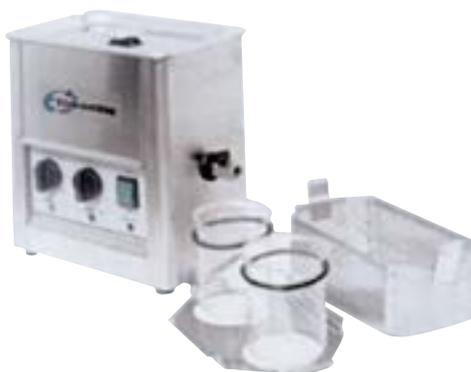
Tank capacity 3,5 litres. With heating. With tap for liquid discharge. With water level indicator. Available accessories: 400 ml pirex beaker, stainless steel beaker holder, stainless steel tray. Overall dimensions: 30W x 17D x 30H cm. Tank dimensions: 23,5W x 14D x 12H cm. Weight 5 kg. Input voltage 230 V ac 50/60 Hz.
