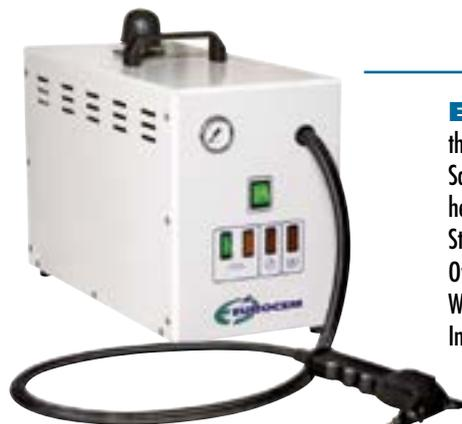
**EGV 14** - Manual loading steam generator. 4 bar working pressure with visualization of the pressure inside the boiler on the pressure gauge. Steam function through gun. Low tension steam outlet control on the gun. Safety devices: double pressure switch and safety valve. Control minimum water level inside the boiler with heater deactivation and pilot light indicating lower water level in the boiler.
