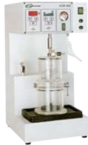
**ECM 400** - Mixer for plasters and investments. With integrated vacuum pump (max vacuum -870 mbar). Adjustment of the mixing time by digital timer. Supplied with the base to place the equipment on the bench and with the support to fix it to the wall. Complete with 500 cc bowl (available on request 200 cc bowl and 1000 cc bowl). Speed 400 rpm. Input voltage 230 V ac 50 Hz. Power 140 W. Overall dimensions cm 18 x 24 x 30 H (56 H with base). Weight kg 10 ( kg 12 with base)
